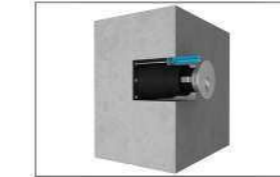
Installation with clips embedded into sleeve, fix on the concrete wall
